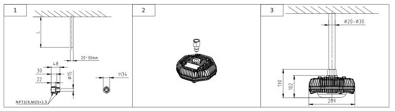
Please use the cable with outer diameter of 7-14mm. The tightening torque of pipe connector is 40N.M.
